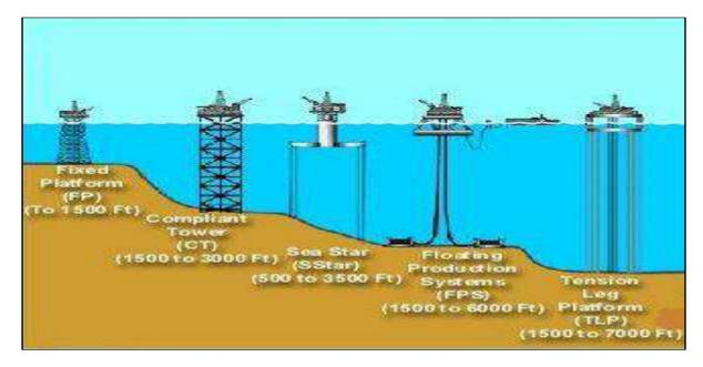
Offshore projects are denoted by offshore facilities for drilling and extracting hydrocarbons. Fixed or floating platforms can be used, depending on water depth. The extracted hydrocarbons are then transported onshore through a sea line-system
